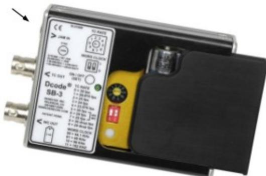
To maintain sync through power cycles we make use of the Denecke SB-3. This device runs on two “AA” batteries and is small enough to attach to the camera while shooting.
