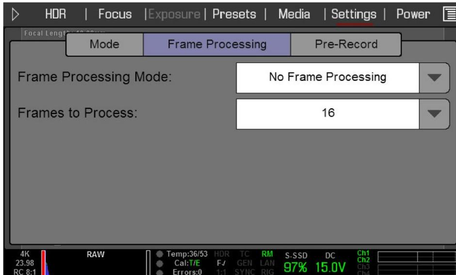
Normal frame processing mode. The FRAMES TO PROCESS selection will not affect your recording.
